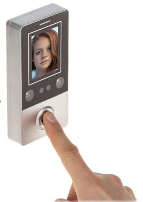
Access controller based on face recognition, fingerprints and RFID cards and key fobs.
