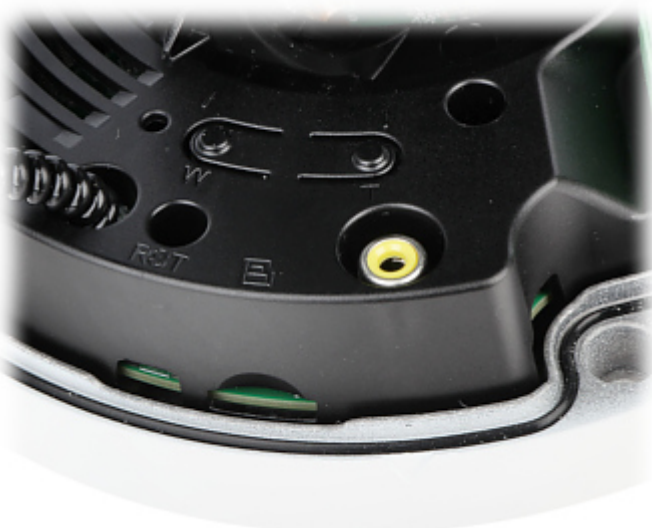
Memory card slot and "Reset" button:
