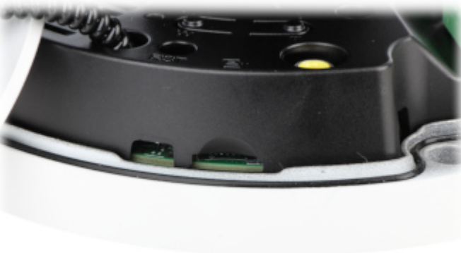
Memory card slot and "Reset" button:
