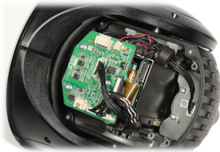
Micro SD card slot is located inside the camera:
