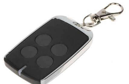
Four-channel remote controller for an automatic gate control.  $% \label{eq:control}%$
