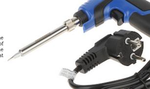
The LUT-0071 pistol soldering iron when connected to the power source heats up and maintains the temperature of the tip at about 200 °C. Pressing the button increases the power consumption to 130 W, thus allowing the tip to heat up to a temperature of up to 450 °C.
