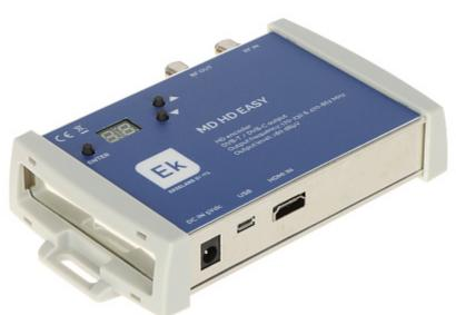
The MOD-EK/DVB-T digital modulator allows to put the HD signal (from camera, terrestrial, satellite TV receiver, Blu-ray, DVD player, etc.) from HDMI input to RF OUT output as DVB-T (COFDM/QAM), Full HD 1080p standard in VHF/UHF bands.
