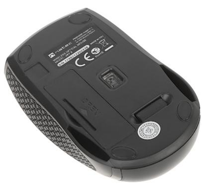
Place for batteries and wireless receiver:
