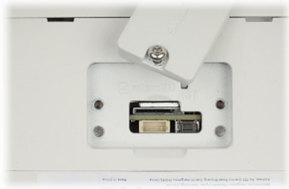
Memory card slot and "Reset" button:
