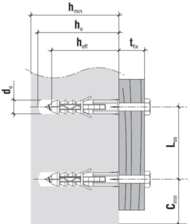
$\begin{array}{l} Hole/drill \ diameter \ [d_0] \ - \ 10 \ mm \\ Min. \ substrate \ thickness \ [h_{min}] \ - \ 90 \ mm \\ Drilled \ hole \ depth \ [h_0] \ - \ 70 \ mm \\ Anchorage \ depth \ [h_{eff}] \ - \ 60 \ mm \\ Max. \ usable \ length \ [t_{fix}] \ - \ 40 \ mm \\ Min. \ axial \ distance \ (concrete/other \ substrate) \ [L_{os}] \ - \ 120/180 \ mm \\ \end{array}$
