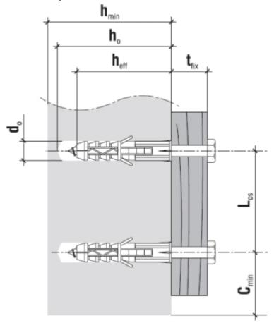
$$\begin{split} & \text{Hole/drill diameter } [d_{\text{o}}] \text{ - } 12 \text{ mm} \\ & \text{Min. substrate thickness } [h_{\text{min}}] \text{ - } 90 \text{ mm} \\ & \text{Drilled hole depth } [h_{\text{o}}] \text{ - } 70 \text{ mm} \\ & \text{Anchorage depth } [h_{\text{eff}}] \text{ - } 60 \text{ mm} \\ & \text{Max. usable length } [t_{\text{fix}}] \text{ - } 20 \text{ mm} \end{split}$$
