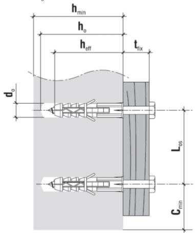
$$\begin{split} & \text{Hole/drill diameter } \left[d_0\right] \text{- }12\text{ }mm \\ & \text{Min. substrate thickness } \left[h_{\min}\right] \text{- }120\text{ }mm \\ & \text{Drilled hole depth } \left[h_0\right] \text{- }90\text{ }mm \\ & \text{Anchorage depth } \left[h_{\text{eff}}\right] \text{- }80\text{ }mm \\ & \text{Max. usable length } \left[t_{\text{fix}}\right] \text{- }40\text{ }mm \end{split}$$
