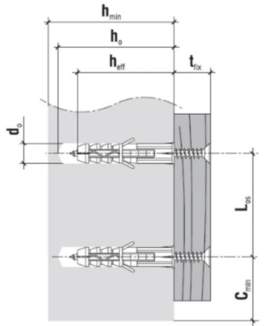
$\begin{array}{l} Hole/drill \ diameter \ [d_o] - 6 \ mm \\ Min. \ substrate \ thickness \ [h_{min}] - 45 \ mm \\ Drilled \ hole \ depth \ [h_o] - 40 \ mm \\ \end{array}$
