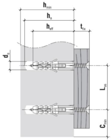
$$\begin{split} & \text{Hole/drill diameter } [d_o] \text{ - 8 mm} \\ & \text{Min. substrate thickness } [h_{\text{min}}] \text{ - 60 mm} \\ & \text{Drilled hole depth } [h_o] \text{ - 50 mm} \\ & \text{Anchorage depth } [h_{\text{eff}}] \text{ - 40 mm} \\ & \text{Max. usable length } [t_{\text{fix}}] \text{ - 20 mm} \end{split}$$
