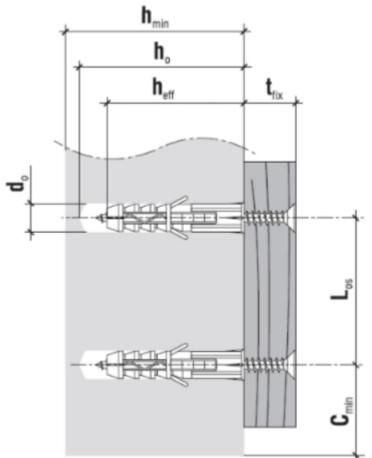
$\begin{array}{l} Hole/drill \ diameter \ [d_{o}] \ - \ 10 \ mm \\ Min. \ substrate \ thickness \ [h_{min}] \ - \ 75 \ mm \\ Drilled \ hole \ depth \ [h_{o}] \ - \ 60 \ mm \\ Anchorage \ depth \ [h_{eff}] \ - \ 50 \ mm \\ Max. \ usable \ length \ [t_{fix}] \ - \ 1 \ mm \\ \end{array}$
