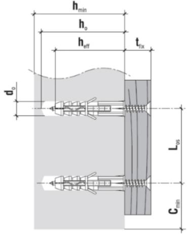
$$\label{eq:hole_drill} \begin{split} & Hole/drill \ diameter \ [d_o] - 10 \ mm \\ & Min. \ substrate \ thickness \ [h_{min}] - 75 \ mm \\ & Drilled \ hole \ depth \ [h_o] - 60 \ mm \\ & Anchorage \ depth \ [h_{eff}] - 50 \ mm \\ & Max. \ usable \ length \ [t_{fix}] - 10 \ mm \end{split}$$
