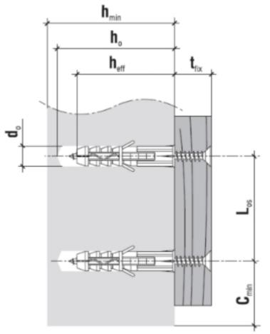
Hole/drill diameter [d\_0] - 10 mm Min. substrate thickness [h\_{min}] - 75 mm
