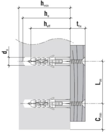
$$\begin{split} & \text{Hole/drill diameter } [d_{\text{o}}] \text{ - 6 mm} \\ & \text{Min. substrate thickness } [h_{\text{min}}] \text{ - 45 mm} \\ & \text{Drilled hole depth } [h_{\text{o}}] \text{ - 40 mm} \\ & \text{Anchorage depth } [h_{\text{eff}}] \text{ - 30 mm} \\ & \text{Max. usable length } [t_{\text{fix}}] \text{ - 5 mm} \end{split}$$
