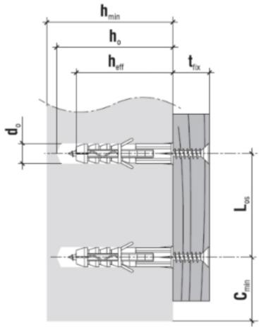
$$\begin{split} & \text{Hole/drill diameter } [d_o] \text{ - 8 mm} \\ & \text{Min. substrate thickness } [h_{\text{min}}] \text{ - 60 mm} \\ & \text{Drilled hole depth } [h_o] \text{ - 50 mm} \\ & \text{Anchorage depth } [h_{\text{eff}}] \text{ - 40 mm} \end{split}$$
