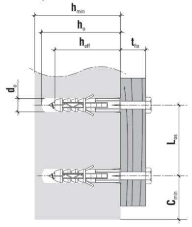
$$\begin{split} & \text{Hole/drill diameter } [d_{\text{o}}] \text{ - } 10 \text{ mm} \\ & \text{Min. substrate thickness } [h_{\text{min}}] \text{ - } 90 \text{ mm} \\ & \text{Drilled hole depth } [h_{\text{o}}] \text{ - } 70 \text{ mm} \\ & \text{Anchorage depth } [h_{\text{eff}}] \text{ - } 60 \text{ mm} \\ & \text{Max. usable length } [t_{\text{fix}}] \text{ - } 1 \text{ mm} \end{split}$$
