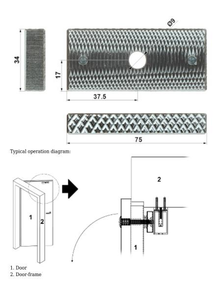
Should pay attention to rubber pads mounted between the door and the movable element of the lock. These pads ensure proper fit the lock elements with the door when it is closed.
