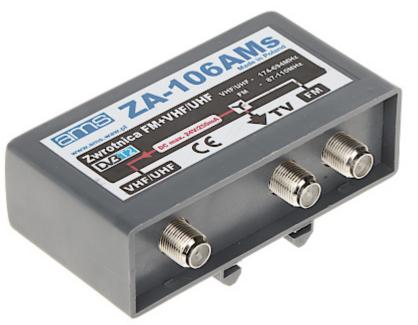
The ZA-106AMS antenna multiplexer with 2 inputs is used as an element combining signals from 2 antennas (receiving signals in FM (87...110 MHz), and VHF+UHF (174...694 MHz) bands), it is installed on the mast carrying the antenna set.
