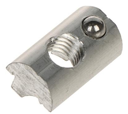
The USP-WPZK sliding groove with ball is used to attach clamps holding solar panels to profiles and mounting rails.
