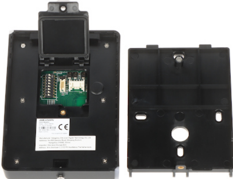
On the body, under the cover there are placed configuration switches
