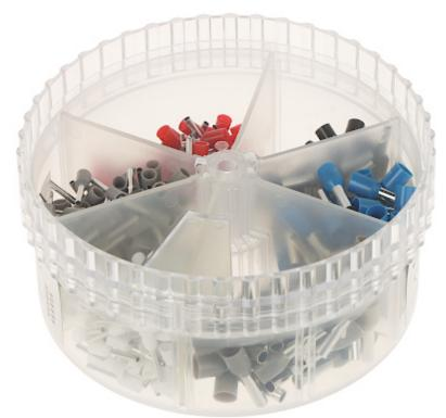
Set of cable ferrules from 0.5  $\,mm^2$  to 4  $mm^2$  with organizer. Cable ferrules are designed for clamping on the stranded wires to keep all loose cable wires together and reduce the risk of a short circuit.
