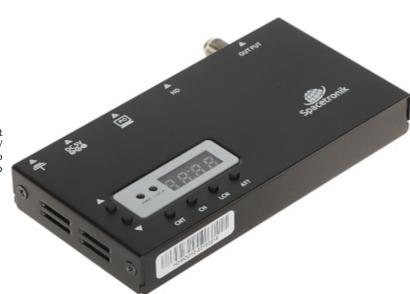
The HDMOD-10/MICRO digital modulator allows to put the HD signal (from camera, terrestrial, satellite TV receiver, Blu-ray, DVD player, etc.) from HDMI input to RF OUT output as DVB-T (COFDM), Full HD 1080p standard in VHF/UHF bands.
