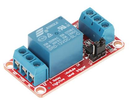
It can be used to increase maximal load of controller transistor output line and for galvanic isolation between output line and load point.
