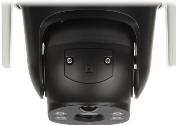
Memory card slot and "Reset" button:
