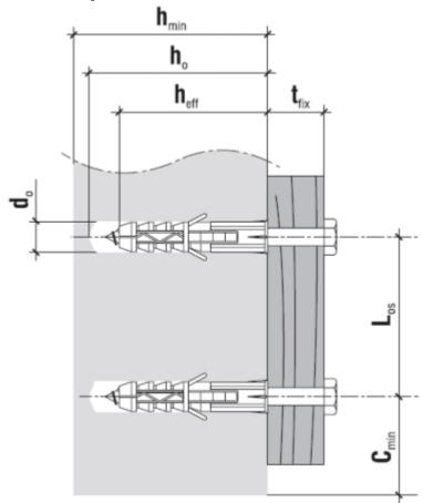
$\begin{aligned} & \text{Hole/drill diameter } [d_0] \text{ - } 14 \text{ mm} \\ & \text{Min. substrate thickness } [h_{\text{min}}] \text{ - } 120 \text{ mm} \\ & \text{Drilled hole depth } [h_0] \text{ - } 90 \text{ mm} \\ & \text{Anchorage depth } [h_{\text{eff}}] \text{ - } 80 \text{ mm} \end{aligned}$
