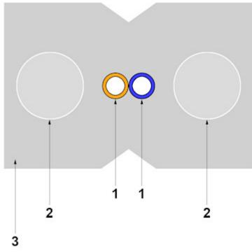
1) Optical fiber in 250  $\mu m$  buffer coating 2) FRP rod
