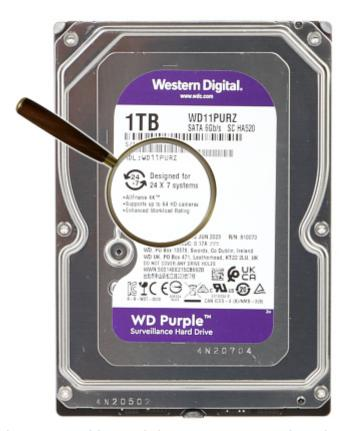
The Western Digital drives marked SURVEILLANCE HDD are designed to work in video surveillance systems. Its design allows for error-free recording of several Full HD streams in 24/7 mode.
