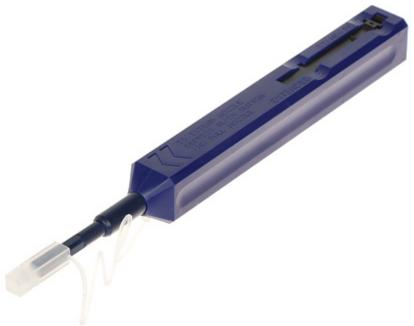
The WUN-XK125 tool is used to clean the end face of the ferrule in fiber optic connectors. A special fabric removes any contaminants, and its antistatic properties prevent dust from settling again. The product is suitable both for cleaning connectors in adapters mounted individually and mounted in patch panels.
