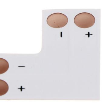
The AD-TL-6499/Z/L connector allows for direct connection of 2 sections of LED strip.
