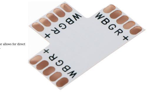
The AD-TL-6499/Z/T/RGBW connector allows for direct connection of 3 sections of LED strip.
