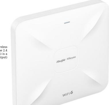
The RG-RAP2260(G) access point broadcasts 2 separate wireless networks in the 5 GHz band with speed 1201 Mb/s and in the 2.4 GHz band with speed 574 Mb/s. The Reyee RG-RAP2260(G) is a device working in 2x2 MIMO (Multiple Input Multiple Output) standard.
