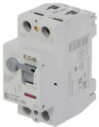
Residual current circuit breaker with rated sensitivity of I $\Delta$ n = 30mA, AC type. The HNC-40/2/003 circuit breaker is compatible to DIN TS-35 rail mounting system.
