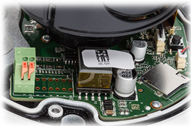
Memory card slot and "Reset" button:
