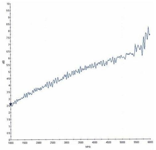
The TRI-LAN-240 cable matching in frequency response:
