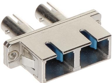
Single-mode hybrid adapter DUPLEX AD-2SC/2ST for connecting two SC type plug with two ST type plugs. Adapters can be easily installed in patch-panels to connect a patchcord with a pigtail spliced to the distribution cable. Mounting holes allow to easy placement the adapter inside patch-panel.
