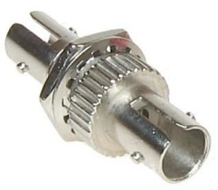
Multi-mode adapter AD-ST/ST-MM for connecting two ST type plugs. Adapters can be easily installed in patch-panels to connect a patchcord with a pigtail spliced to the distribution cable. The threaded body and nut allow to easy placement the adapter inside patch-panel.
