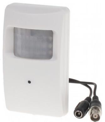
The color camera with SONY sensor and IR illuminator, hidden in dummy PIR (without the real PIR).
