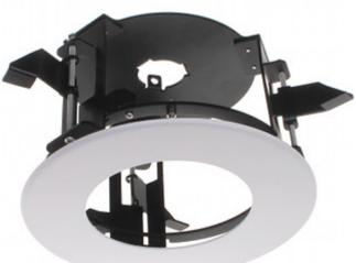
Suspended ceiling bracket. Designed to OWA type ceilings. Bracket with camera is freely placed on the suspended ceiling. Installation needs access to both sides of camera mounting panel hole. The most part of camera is hidden in ceiling, so the camera looks like typical dome camera (due to its small dimensions).
