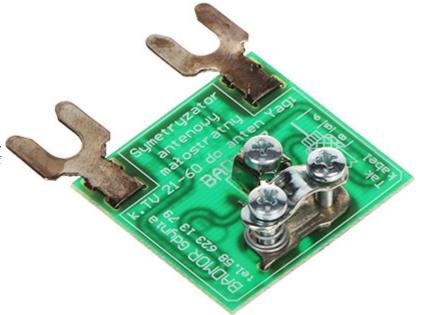
The SA/IV-V-DIPOL antenna impedance transformer matches the antenna impedance to the impedance of coaxial cable.
