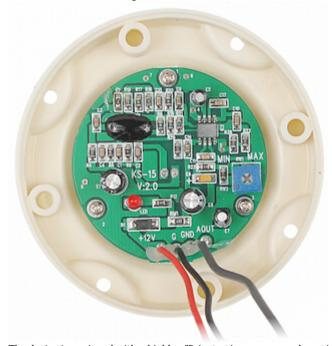
The device is equipped with a highly efficient, microprocessor dynamic compressor that adapts the level of amplification to the ambient noise level. Mounting side view:
