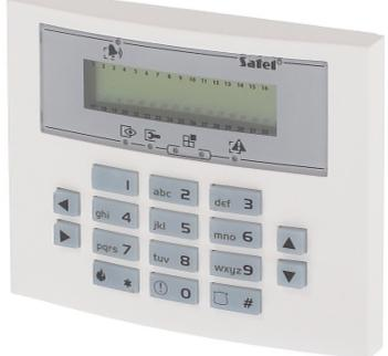
The INT-KLCDS-GR keypad is intended for daily operations and programming the INTEGRA series alarm control system. With the LCD display showing text messages, even advanced functionalities of the alarm control unit are simple and convenient.
