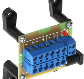
The LZ-1ML is a passive device and allows to distribute the power
