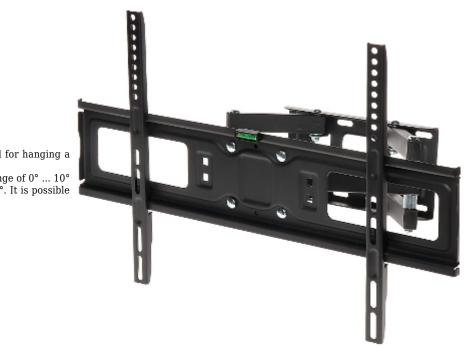
The AX-TYTAN-MAXXIM mount is intended for hanging a TV or LCD / OLED monitor on the wall. It allows to easy adjustment of tilt in the range of  $0^{\circ} \dots 10^{\circ}$  and horizontal rotation in the range of  $\pm 90^{\circ}$ . It is possible to rotate the plane of the screen  $\pm 3^{\circ}$ .
