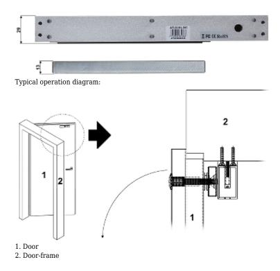
Should pay attention to rubber pads mounted between the door and the movable element of the lock. These pads ensure proper fit the lock elements with the door when it is closed.
