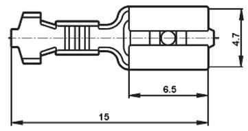
Female connector and suitable male connector:
