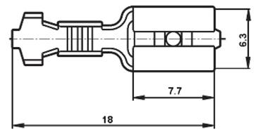
Female connector and suitable male connector:
