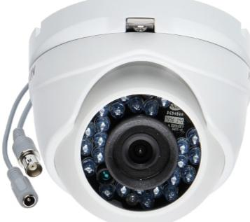
Megapixel camera with 1/2.7" CMOS sensor and HD-TVI (High Definition Transport Video Interface).
